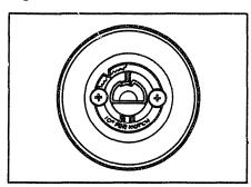
1. Pull off knob, loosen both screws on back of knob holding skirt of knob firmly. 2. Turn black handle to move pointer one notch in desired direction. Tighten screws.
